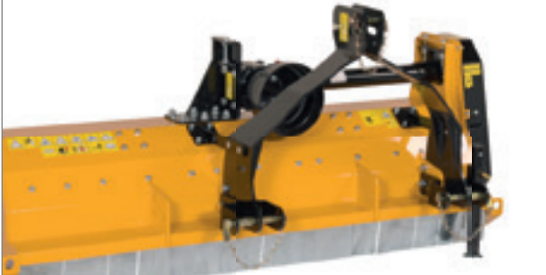
The headstock of the MU-ECOTOP can be unbolted and moved behind the tractor and offset to the side.
