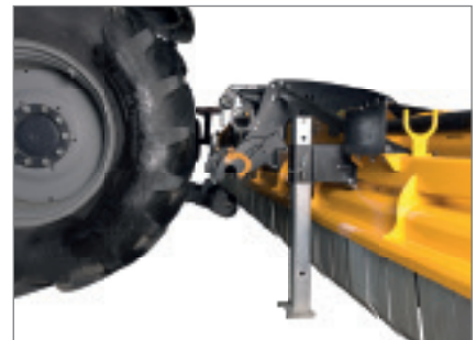
Quickly ready for operation: Uncouple the machine and bring the lengthways transport device into the work position / couple the MU-Farmer® 670 to the tractor with the quick coupling bar and connect the PTO shaft.
