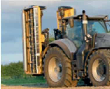
Short design for a centre of gravity close to the tractor (quick hitch-suitable).
