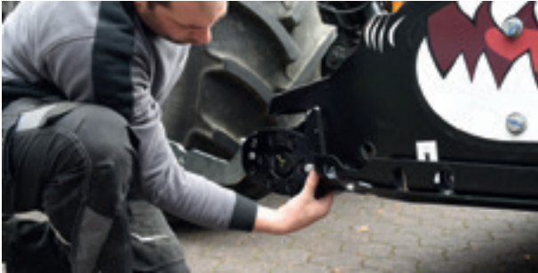
Easy adjustment of the swivelling support roller even without additional help.
