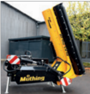
A clever design allows the flail mower to be folded up for space-saving storage.
