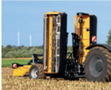
The hydraulically adjustable working and transport position ensures a transport height of less than 4 m.
