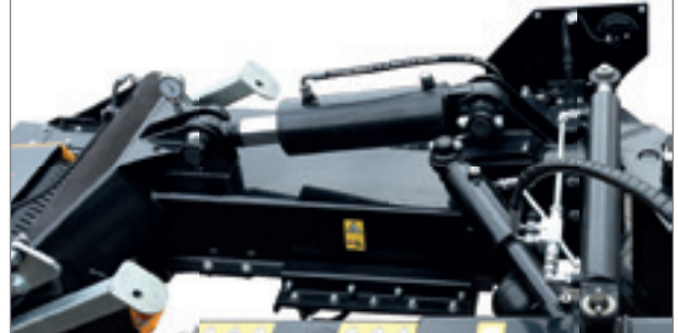
Hydropneumatic weight transfer system for optimal ground adaptation.
