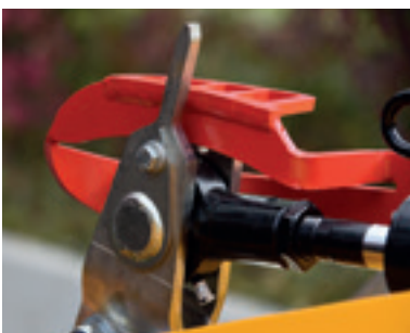
The Vario-Shift adjustable hydraulic cutting bar enables fast, infinitely variable adjustment of the shredding rate to the respective requirements directly from the driver's cab (optionally available for MU-PRO Vario 280).
