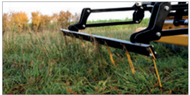
Insect rescuer: A specially designed, hydraulically folding bracket with integrated angled tines frightens away insects and small organisms from the front of the flail mower and causes them to flee. (optional for working widths of 1,60 m and 2.20 m)
